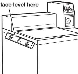
Place level here
