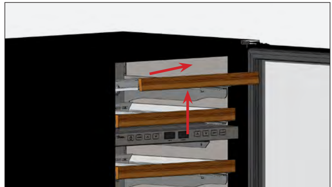
FIG. 1. Lift and pull the wine rack forward.
