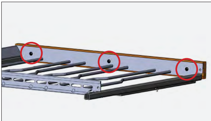
FIG. 2. Wine rack handle screw locations.
