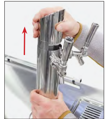
FIG. 5. Lift the top off the draft standard.
