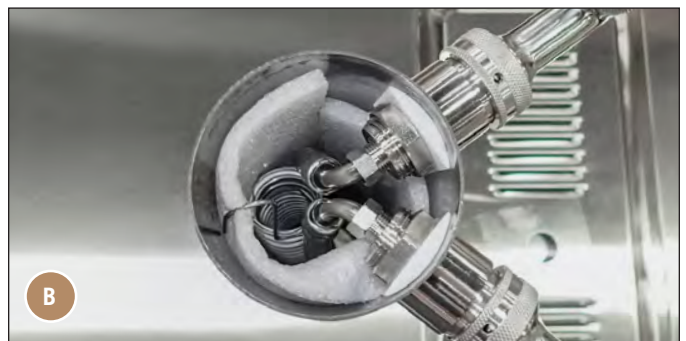
FIG. 6. Route the chill hose into the draft standard from below (A) and hook it on the top of the insulation sleeve (B).
