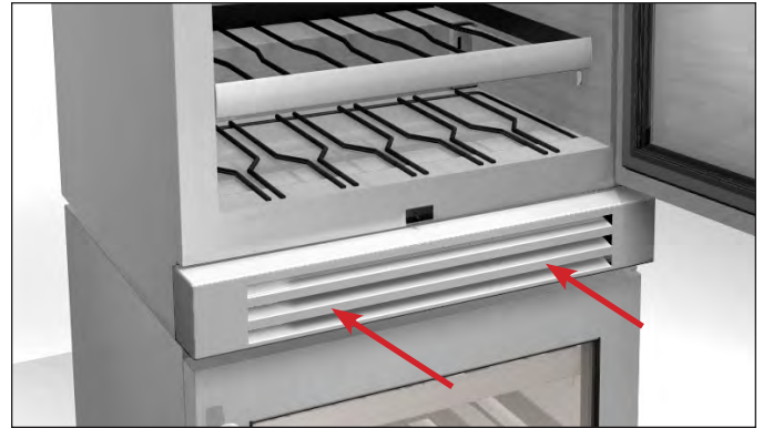
FIG. 4. Position the provided grill.
