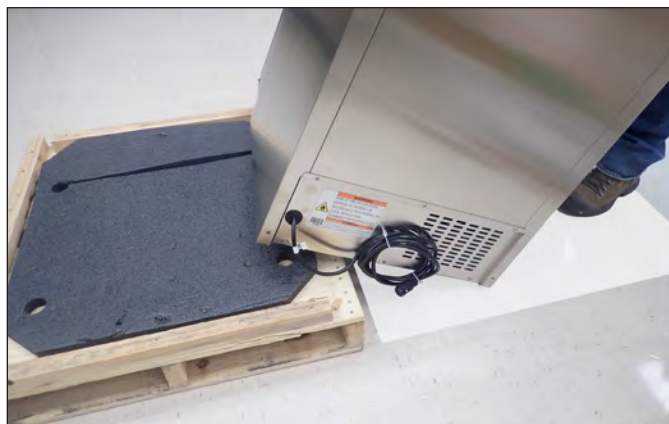
FIG. 3. Get the unit off the skid from the side.
