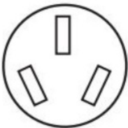
3-wire receptacle (10-50R)
